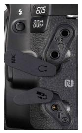
**External microphone.** There are lots of accessory microphones that you can use to record sound that syncs with the video. For interviews, we'd like you to use a small lavalier mic that clips to the speaker's collar and then plugs into the cameras audio in port on the left side of the camera.
